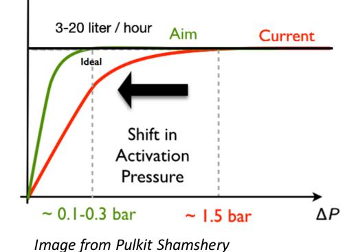
**Reducing the activation pressure**, or minimum functional pressure of drippers allows for smaller pump and smaller systems, and can halve system
